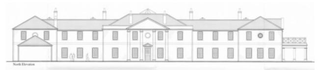
Fig. 3: Proposed northern (rear) elevation, incorporating the main entrance
